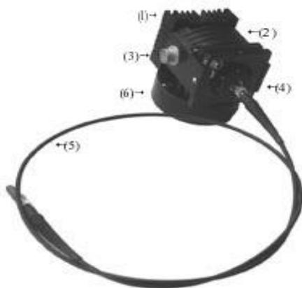
Fig 3. Miniaturized fibered MCT photo-receiver: (1) – heat-sink; (2) case containing PC MCT MWIR TE cooled detector, plate with changeable filter and focusing lens, (3) – electrical connectors on both sides of the case; (4) – adjustable optical unit with optical SMA connector; (5) – optical fiber cable and (6) – preamplifier box. Overall dimensions: Length x Width x Height – 87,5 x 66,0 x 70,5 mm
