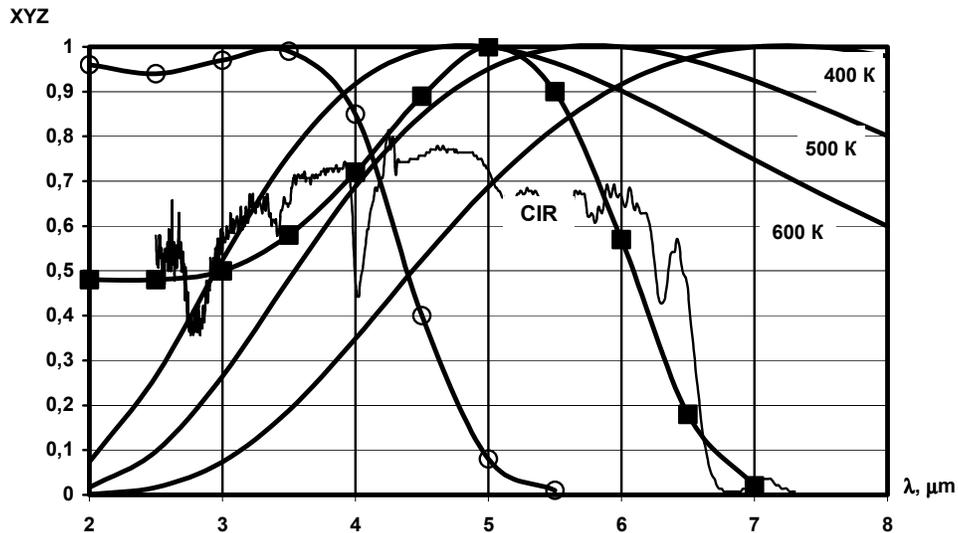
Fig. 5. “X” – normalized photon power radiant flux density (black body  $T = 400, 500$  and  $600$  K); “Y” – spectral responsivity curves of Mid-Wave MCT detectors; and “Z” – spectral transparency of 1 meter long CIR fiber with core diameter  $1000 \mu\text{m}$  (absolute value)
