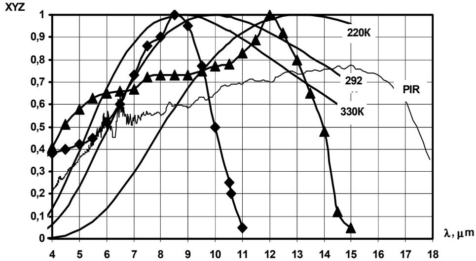
Fig. 7. “X” – normalized photon power radiant flux density (black body  $T = 220, 292$  and  $330$  K); “Y” – spectral responsivity curves of Long-Wave MCT detectors; and “Z” – spectral transparency of 1 meter long PIR fiber with core diameter  $1000 \mu\text{m}$  (absolute value)
