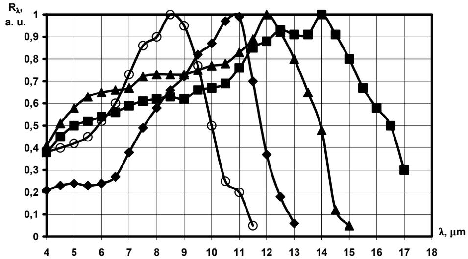
Fig. 6. Typical spectral responsivity curves of liquid nitrogen cooled fast MCT photoconductive infrared detectors. Spectral response is varied with MCT composition “x” and is optimal for coupling with PIR-fibers
