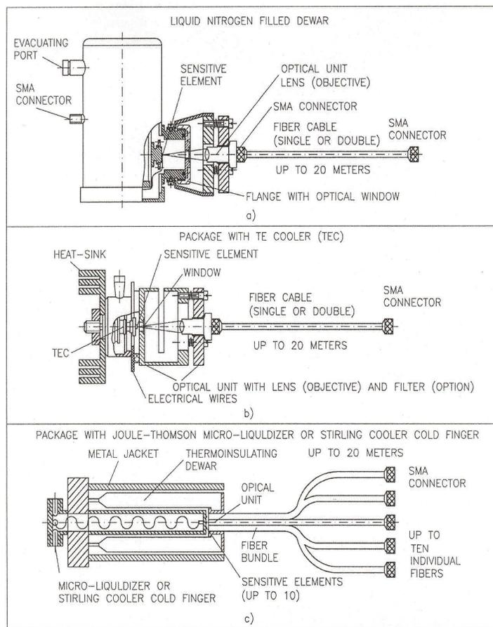
Fig.2. Design concept of MCT infrared radiation detectors with fiber input:
