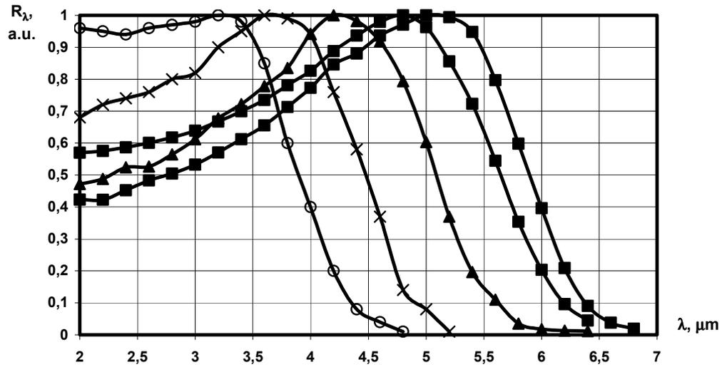
Fig. 4. Typical spectral responsivity curves of thermoelectrically cooled MCT photoconductive infrared detectors. Spectral response is varied with MCT composition “x” and is optimal for coupling with CIR-fibers
