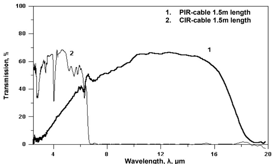
Fig.1. Typical transmission spectra of CIR-fiber cable 750/850  $\mu\text{m}$  Core/Clad diameters and PIR-fiber cable 900/1000  $\mu\text{m}$  Core/Clad diameters both with length of 1,5 meter
