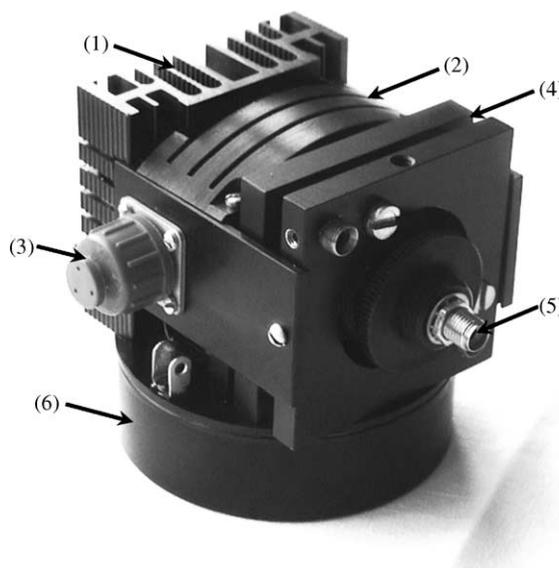
Fig. 4. Miniaturized fibred MCT photo-receiver: (1) heat-sink; (2) case containing PC MCT MWIR TE cooled sensor and plate with changeable filter (option); (3) electrical connectors on both sides of the case; (4) optical coupler with optical SMA connector; (5); and (6) preamplifier box. IR-fibre cable is detached. Overall dimensions: length, 87.5 mm; width, 76.0 mm; height, 70.5 mm.
