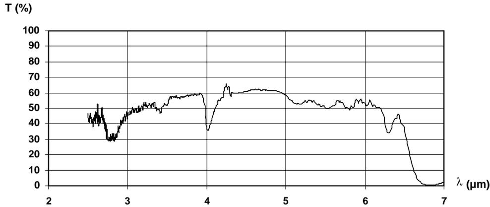
Fig. 1. Spectral transparency of 1 m long CIR-fibre with core diameter 1000  $\mu\text{m}$  (absolute percentage).
