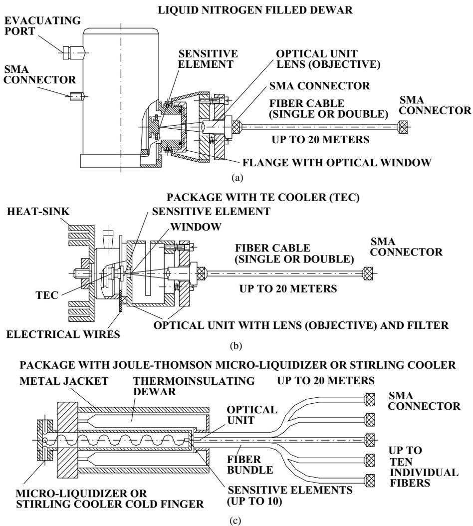
Fig. 3. Design concept of fibre coupled MCT infrared radiation detectors: (a) and (b): design with outside detachable optical coupler and (c): design with fixed optical coupler.
