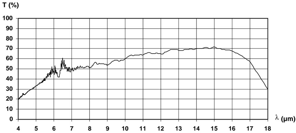
Fig. 2. Spectral transparency of 1 m long PIR-fibre with core diameter 1000  $\mu\text{m}$  (absolute percentage).
