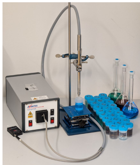
Figure 1. Measurement setup with a transfection fiber-optic probe (art photonics GmbH) with an adjustable optical path length.
