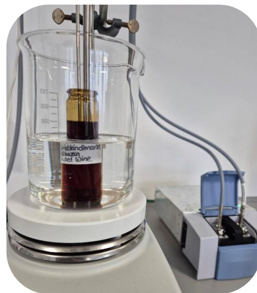
Figure 1. Exemplary Laboratory Setup with Bruker Alpha spectrometer with inserted Fiber Coupler and Diamond ATR Fiber Probe.
