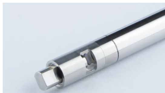
Figure 2. Transfection probe tip for the NIR-spectroscopic analysis of ethanol-methanol mixtures.
