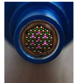
Mixed fiber bundle consisting of UV silica, VIS-NIR silica and CIR fibers to enable remote spectroscopy in 0.2 \mu\text{m} to 6 \mu\text{m} spectral range
