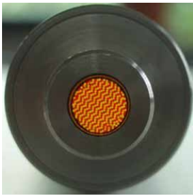
Coherent and randomized silica fiber bundle
