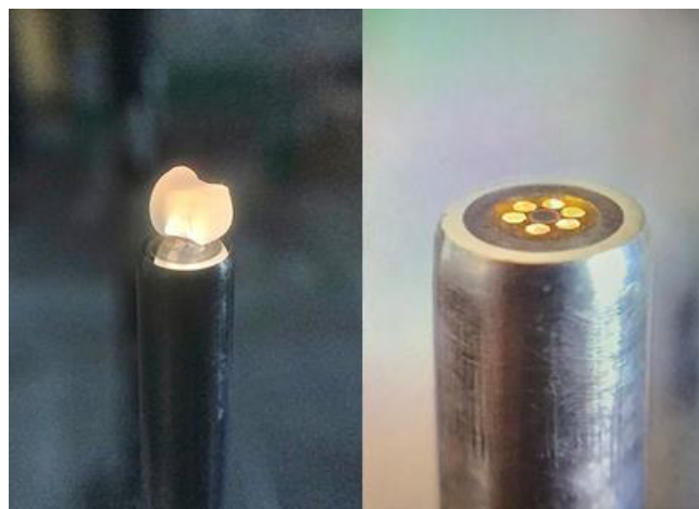
Figure 1. A polymer granule placed at the fiber probe tip (left) and the probe with six illuminating and one detecting channel (right).
