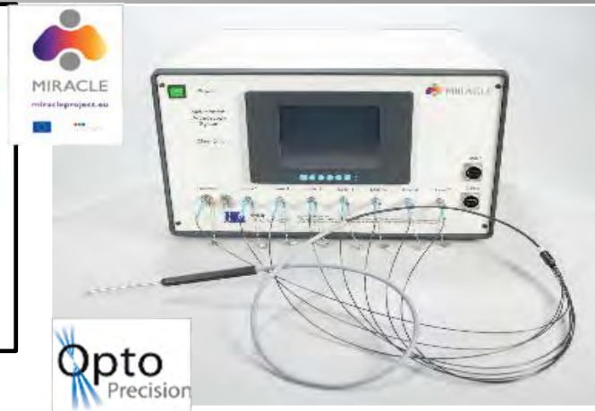
PIR-fiber bundle combines radiation of 7 QC-Lasers into Arthro-Probe
