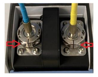
Loose these screws for Z-axis alignment. Move the part with SMA-connectors carefully up and down approx. 0,5-1mm for maximal signal. Tighten screw after. Align the connectors one separately from the other.
