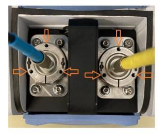
Rotate these screws for Angle alignment. Each screw regulates the height of the SMA-unit in this position. Align the screws one separately from the other.
