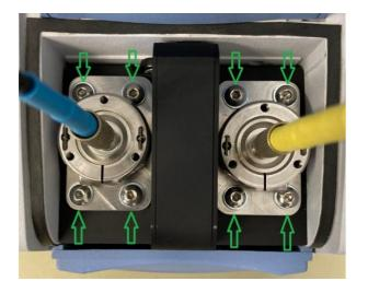
Loose these screws for X-Y-axis alignment. Move the whole part with SMA-connectors carefully approx. 0,5-1mm for maximal signal. Tighten all screws after. Align the connectors one separately from the other.
