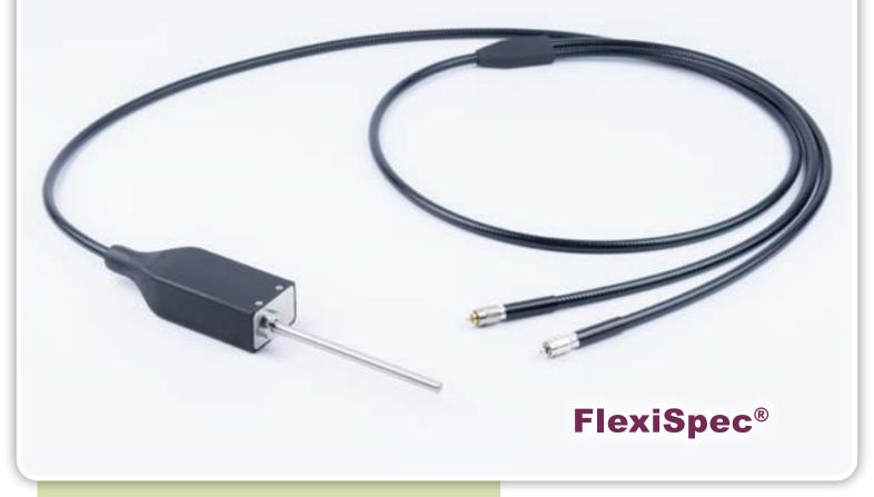
**FlexiSpec®** Raman fiber optic probes, compatible with any Raman spectrometer, come in multi-wavelength (630-785 nm) and single-wavelength (532, 785 nm) options. Their bifurcated design connect to both a laser and a spectrometer, enabling analysis in the fingerprint (800-1800 cm<sup>-1</sup>) and high wavenumber (2800-3800 cm<sup>-1</sup>) ranges. These probes are designed for reaction monitoring in labs and pilot plants.
