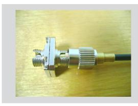
Take care to insert the cable into the FC/PC adapter properly according the position key as shown in the photo
