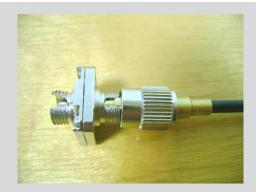
Take care to insert the cable into the FC/PC adapter properly according the position key as shown in the photo!
