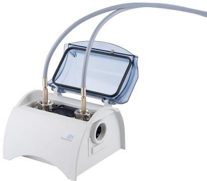
FPC-2M design is based on two off-axis parabolic mirrors inside the standard accessories iD1 which can be adjusted for maximum signal from SMA-terminated probe. These enable efficient coupling of fiber probes to Nicolet™ Summit FTIR, Nicolet™ iS™ 5 and Nicolet™ iS™ 5N FT-NIR Spectrometers (Thermo Scientific™) when installed in its sample chamber.
