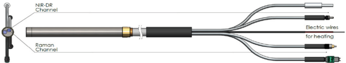
Fig.1 NIR-DR + Raman Combi Probe is a multichannel fiber optic probe designed for in situ NIR diffuse reflectance (NIR-DR) and Raman measurements of powders or liquids. NIR-DR and Raman channels of the probe can work simultaneously – the wavelength ranges of both channels are separated: Raman 785 – 1000nm; NIR-DR 1000-2500nm. The probe shaft is electrical heated to prevent moisture conden-
