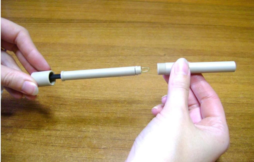
Screw on and tighten the screw nut. Rotate the nut but not the cap.
