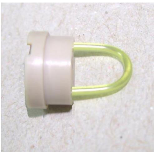
Prevent any contamination of the fibre ends on the probe tip. Take care not to lose Teflon sealing ring (inside the fixing cap).
