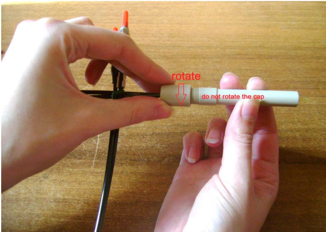
Take the old loop from the slot on the probe and prepare a new loop tip.
