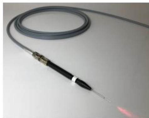
Figure 1: Left: Human tongue tissue samples: cancer tissue marked with the red pins, surrounded by healthy tissue marked with the green pins. Right: “Raman – needle” fiber optic probe.
