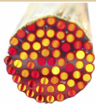
Soldered MCS fiber bundle for combining power up to multi-kW range from many diode lasers.
