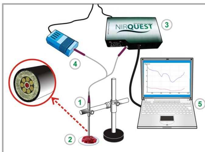
Figure 1. Setup for NIR measurements. (1)-NIR probe R(1+7) from art photonics GmbH<sup>13</sup>, (2)-Tissue slice in petri dish, (3) NIRQuest spectrometer, (4)- halogen lamp, (5)- PC with software for spectra collection
