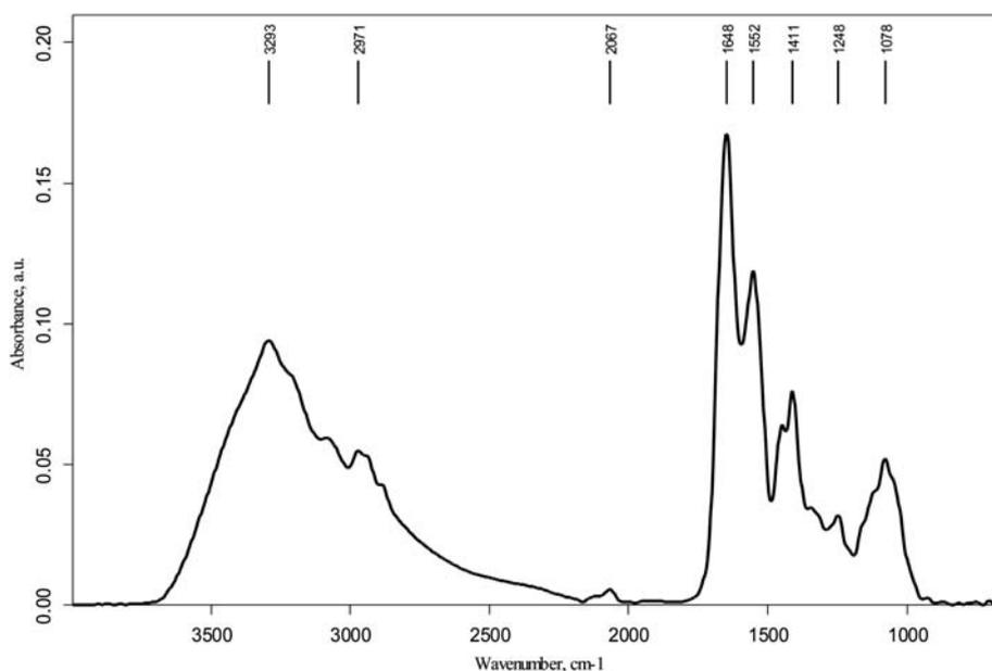
**Fig. 2** Averaged spectrum of saliva recorded in 4000–600  $\text{cm}^{-1}$  region. The main absorption bands are marked.
