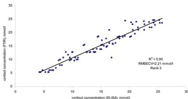
**Fig. 5** Cortisol concentration in saliva. Correlation between the cortisol concentrations obtained by FTIR spectroscopy and ELISA.
