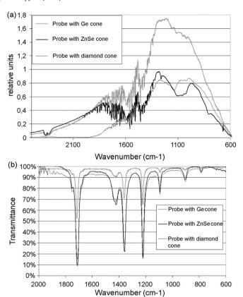
**Fig. 3.** Background (a) and acetone transmission (b) spectra obtained using ATR-probes with two-bounce cone optical element made of different materials.
