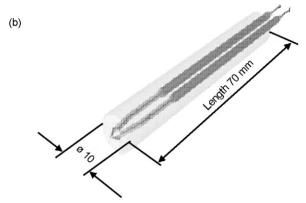
Fig. 1. Appearance (a) and design (b) of fibre probe tip with ATR cone element.
