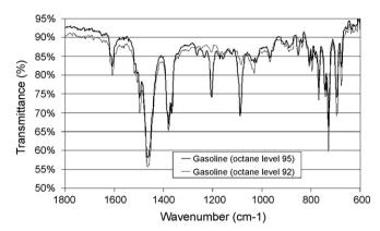
Fig. 7. Transmission spectra of different kinds of fuel.
