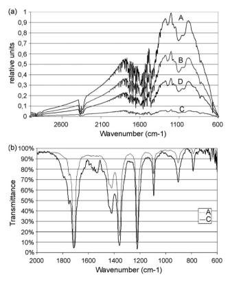
**Fig. 4.** Background (a) and acetone transmission (b) spectra obtained using ATR fibre loop probes with different shaped loop tips.
