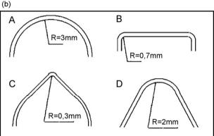
**Fig. 2.** Appearance and design of fibre probe tip with detachable loop ATR element (a). Disposable fibre loops of different shape (b): standard U-shaped (A), "rectangle" (B), "triangle" (C) and V-shaped (D).
